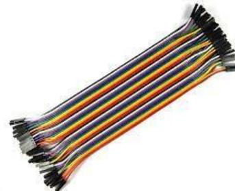
Jumper wires typically come in three versions: male-to-male, male-to-female and female-to-female. The difference between each is in the end point of the wire. Male ends have a pin protruding and can plug into things, while female ends do not and are used to plug things into.
