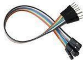
Jumper wires typically come in three versions: male-to-male, male-to-female and female-to-female. The difference between each is in the end point of the wire. Male ends have a pin protruding and can plug into things, while female ends do not and are used to plug things into.
