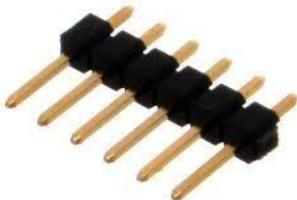
Male pin headers are often associated with ribbon cable connectors. When used alone, they can be recipients of jumpers, which have spacings of 2.54 mm (0.1 in) and 2.00 mm (0.079 in). The spacing distance between pins (measured from center to center) is often known as pitch.
