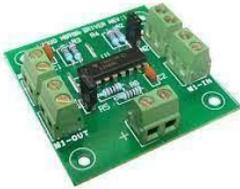
L293D is a basic motor driver integrated chip (IC) that enables us to drive a DC motor in either direction and also control the speed of the motor. The L293D is a 16 pin IC, with 8 pins on each side, allowing us to control the motor. It means that we can use a single L293D to run up to two DC motors. L293D consist of two H-bridge circuit. H-bridge is the simplest circuit for changing polarity across the load connected to it.
