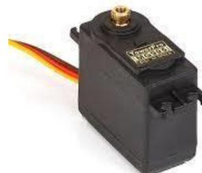
MG995 Metal Gear Servo Motor is a high-speed standard servo can rotate approximately 180 degrees (60 in each direction) used for airplane, helicopter, RC-cars and many RC model. Provides 10kg/cm at 4.8V, and 12kg/cm at 6V. It is a Digital Servo Motor which receives and processes PWM signal faster and better. It equips sophisticated internal circuitry that provides good torque, holding power, and faster updates in response to external forces. Features and Electrical Characteristics:
